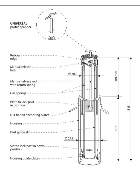
GASPO 252 is a manually operated post for traffic control consisting of a cylindrical post made of steel, having a diametre of 200 mm and a height of 500 mm.
