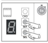
1 • Press the SEL and SET buttons simultaneously for 5 sec. to access the programming menu.
