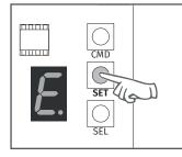
3 • Press the **SET** button to access the submenu.
