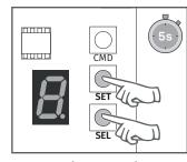
1 • Press the SEL and SET buttons simultaneously for 5 sec. to access the programming menu.
