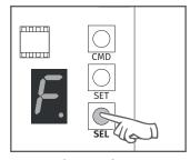
2 • The display will show F. Press the SEL button as many times as necessary until the display shows H.
