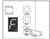
2 • The display will show F. Press the SEL button as many times as necessary until the display shows L.
