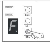
2 • The display will show F. Press the SEL button as many times as necessary until the display shows E.
