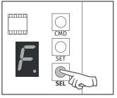
2 • The display will show F. Press the **SEL** button as many times as necessary until the display shows **P**.
