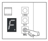
2 • The display will show F. Press the **SEL** button as many times as necessary until the display shows **A**.
