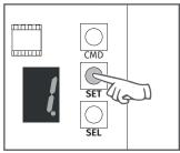
4 • Use the SEL button to put on the desired option. Press the SET button once to save this option.
