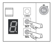
1 • Press the SEL and SET buttons simultaneously for 5 sec. to access the programming menu.
