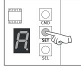
**3 •** Press the **SET** button to access the submenu.
