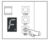
2 • The display will show F. Press the SEL button as many times as necessary until the display shows C.
